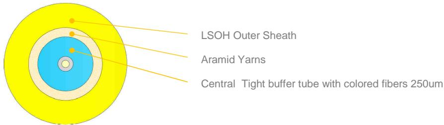
\*Schematic drawing, not in scale
