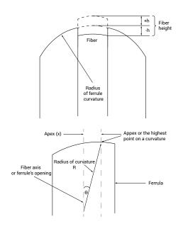
Therefore, the connector is wearing, which generates extra costs for its maintenance. What is even worse, an extended radius of curvature inhibits the physical contact so the return loss is decreasing drastically!
