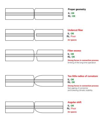
If the value of this parameter exceeds the norms, it will result in shorter work longevity and significantly lower connector's stability!
