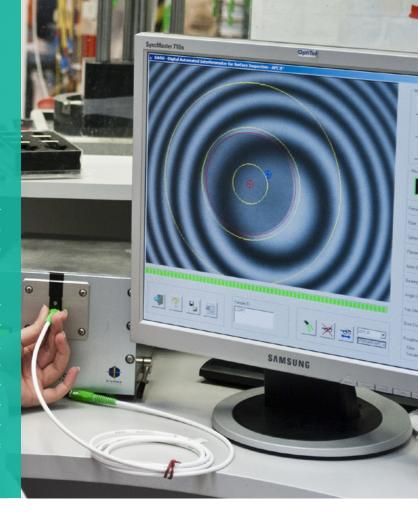
When it comes to network design, we need to remember about a few important aspects. To begin with, Insertion Loss (IL) and Return Loss (RL) are crucial parameters which determine the quality and the ferrule's class. No to mention that it is the ferrule, which is the core component of each fiber optic connector. An optical fiber is placed in its opening, and then ferrule with a fiber is carefully polished.
